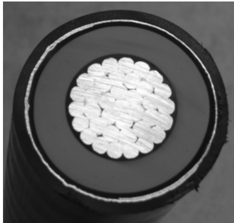
Figure H230-3 Metal-sheathed cable meeting Rule 230C1a
